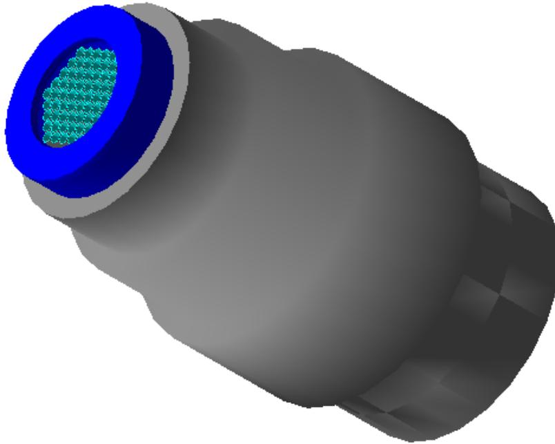
Figure 2.1: PoGOLite as rendered by the polaripogo simulation software. The grey enclosure is a polyethylene neutron shield discussed in [14, 19], the blue cylinder is the pressure chamber that houses the polarimeter, and the cyan hexagonal tubes are the PDCs.
